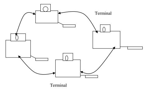
Each node is connected to two (2) others forming a ring.
