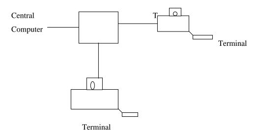
A number of small computers or peripheral devices are linked to a central unit. The central unit may be a host computer or a file server.
