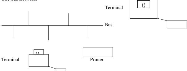
In the bus network, each device handles its own communication control. There is usually no host computer or file server.
